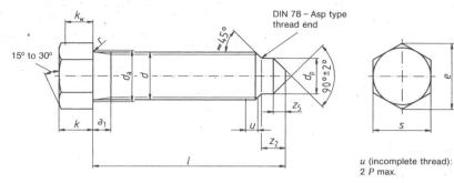
$k_{\rm w}$  is the minimum wrenching height; e shall be maintained within  $k_{\rm w}$ .  $a_1$  as in DIN 76-1,  $d_{\rm p},z_2$  and  $z_5$  as in DIN 78.
